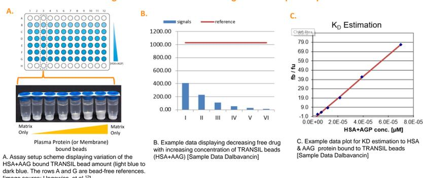
Figure 6: TRANSIL HSB Kit Design and Example Output Data
